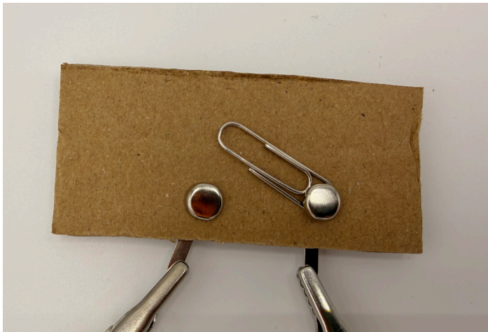
Above: The switch is open
