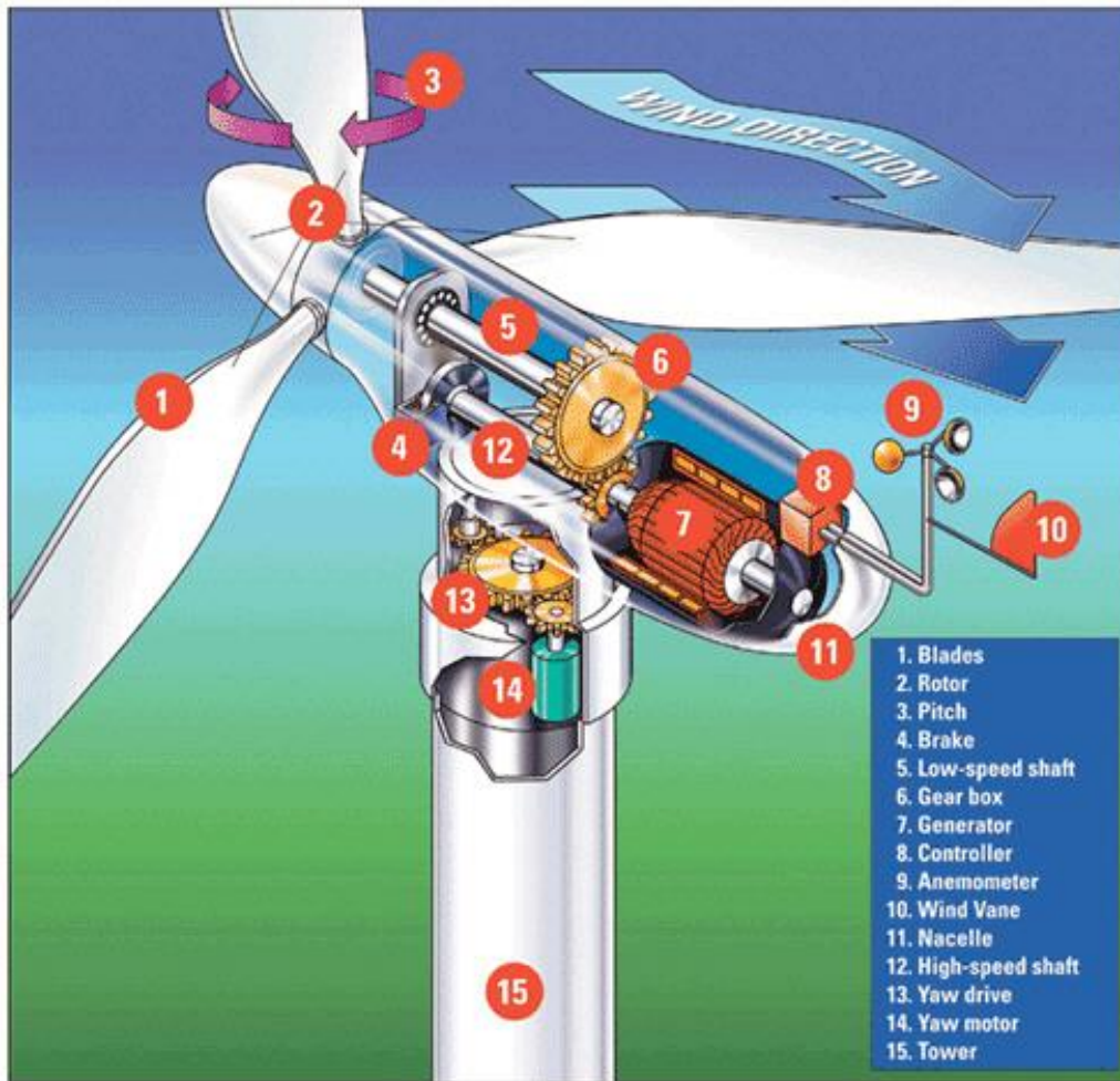
Figure 5. A wind turbine – an inside view.
